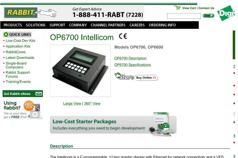
The Intellicom is a C-programmable, 12-key graphic display with Ethernet for network connectivity and a VFD option for applications requiring high visibility. To accommodate users' installation preferences, the versatile Intellicom can be either wall or panel mounted.
